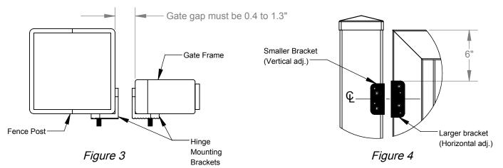
3. Install self-closing hinge assembly to mounting flanges (installed in step 2) and secure with washers and acorn nuts (USE HAND TOOLS ONLY). Hinge should be positioned as shown so that the locking grooves on the mounting flanges will align with grooves on the back side of the hinge assembly (Figure 5).
